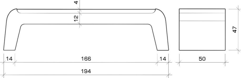
Technical drawing of a concrete bench with wooden slats. Dimensions shown: height 47, backrest height 12, seat height 4, width 166, depth 50, and side height 14.
