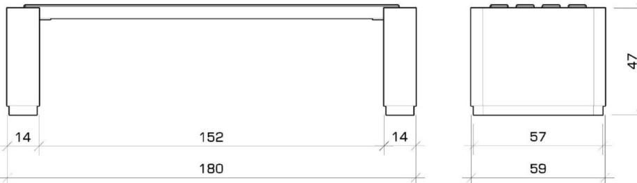
Technical drawing of a concrete bench with wooden slats. Dimensions shown: height 47, backrest height 14, seat height 14, width 180, depth 59, and side height 152.
